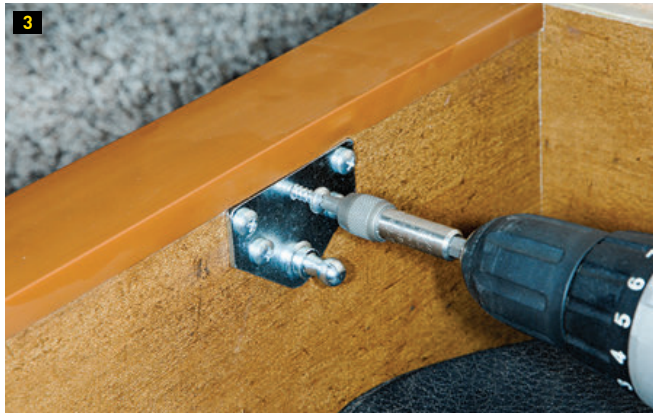
3) The bottom bracket is installed using wood screws. Here, there was plenty of wood backing to facilitate a strong connection. 4) Gas struts are snapped on the ball ends of the upper and lower brackets.
