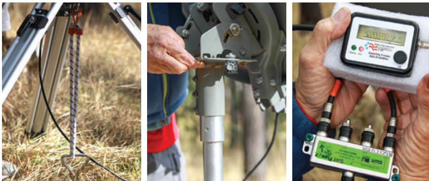
(Below from left) The heavy-duty bungee cord and tie-down stake secure the tripod in even the softest of dirt. Carefully set the dish onto the mast for the initial setup and follow the directions. H&G's custom signal finder eliminates the need for the help of another person during the aiming process.
