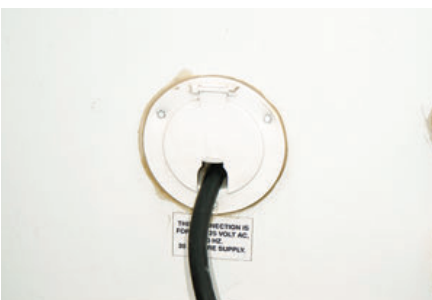
(Above from left) The original power cord hatch cannot be locked. The Fortress PowerLock is designed to prevent access to the cord by completely covering the hatch.
