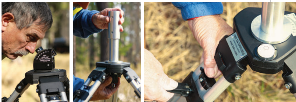
(Above from left) Set the degrees of elevation, and this custom aiming scope will enable you to check for obstructions in the line of sight. A solid aluminum machined mast is designed to fit a 1½- or 2- inch bracket as well as supporting up to 35 pounds. The tripod has an infinite amount of adjustment for each leg, thus making the leveling process fast and easy.
