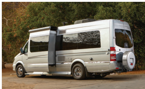
(Above left to right) Cockpit is well laid out with shelves and pockets for keeping road-trip widgets within reach. Streetside slideout houses the couch/sofa bed and adds 25 inches to the floor space.
