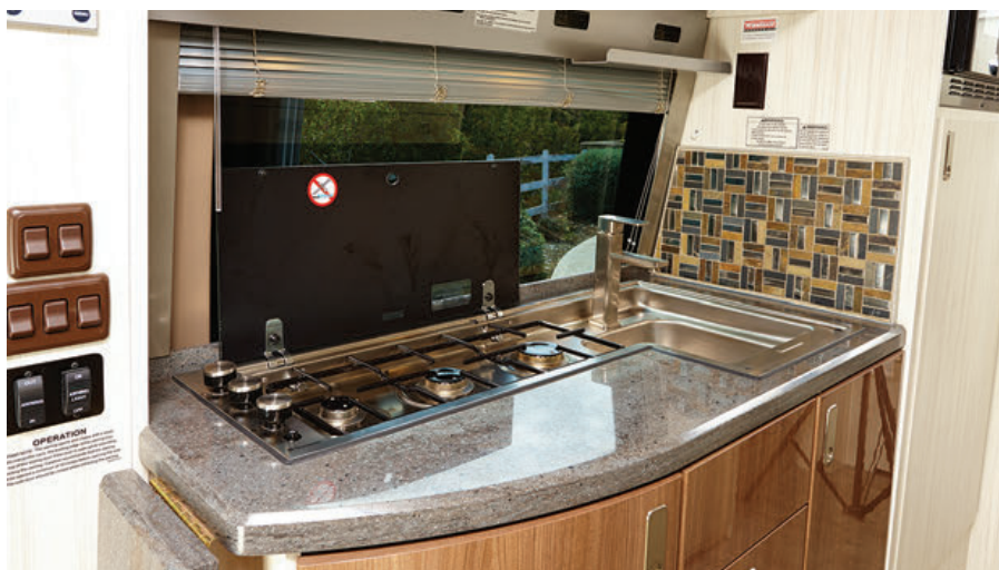
Galley layout is practical with flip-up countertop extension (shown down), three-burner range with glass top and deep stainless-steel sink. Elegance is added with a curved Corian countertop and attractive backsplash.
