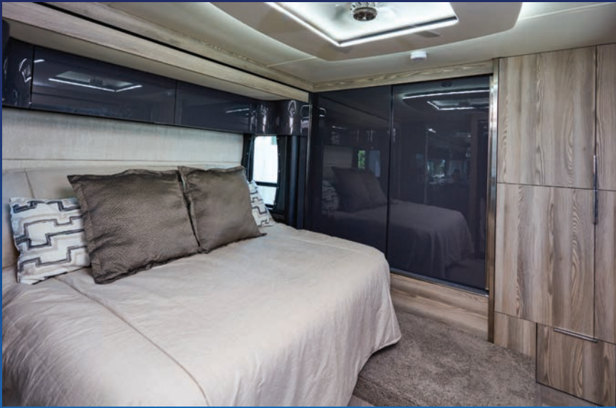
King bed must be collapsed (using electric motor) to make room when the slideout is retracted. Wardrobe closet is large and configured well adjacent to the washer/dryer cabinet.
