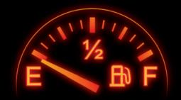
is faulty. The gauge is probably OK, because it sweeps through its full scale. It's likely that either the sending unit is faulty, or the wire connecting it to the gauge has been chafed. I would start by checking the wiring and connections by the gas tank. If the tank has to be removed to access the sending unit, make sure to drive the motorhome until the tank is almost empty.
