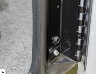
you will also need some basic hand tools such as a wrench, screwdriver, pliers and maybe a socket wrench. These items will be needed to tighten the hinges and the cargo-door mounting bolts, and to adjust anything that is not perfectly aligned. This is a very easy project that should take no more than one or two hours, and if you work in the shade you will never even break a sweat.
