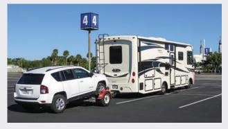
sates for the weight of the vehicle when braking hard. Therefore, my recommendation is that a tow dolly is a good solution when towing a not-too-heavy front-wheel-drive vehicle behind a motorhome in areas that are not too mountainous.
