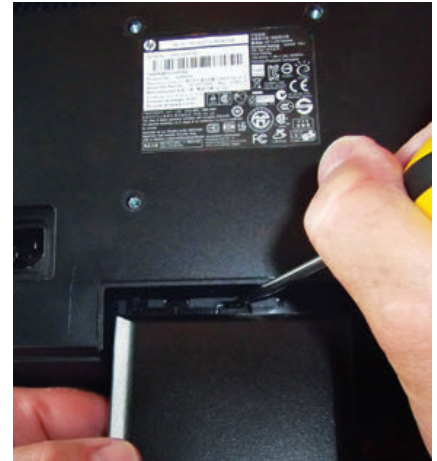
7. Remove the desktop mounting from the monitor or all-in-one PC.
