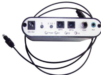
The digital sound decoder for this project is shown with the included power supply and one short TOSLINK fiber cable.
