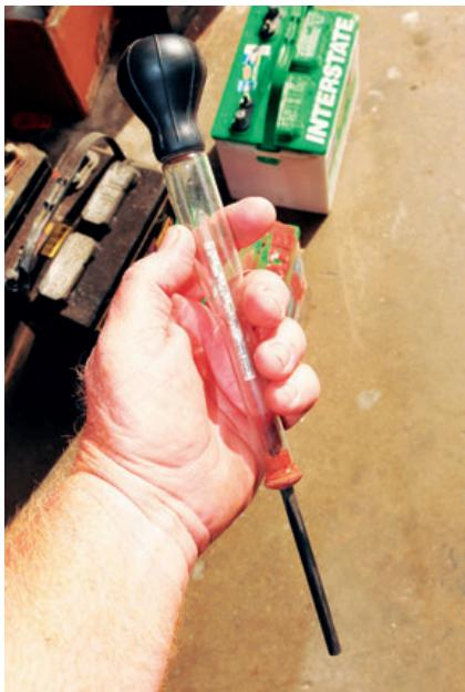
A hydrometer is an easy and inexpensive way to check the health of an open-cell battery. Simply insert the tube into a cell, squeeze and release the bulb, and electrolyte (water) is drawn into the hydrometer's chamber. Ideally, the specific gravity number should be 1.265 to 1.275 when fully charged. Repeating this process in each cell will help determine if there are any weak or dead cells. Temperature-correcting hydrometers (not shown) are best.
