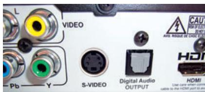
On a DISH receiver, the optical fiber connection is labeled Digital Audio Output. It accepts the TOSLINK fiber cable.
