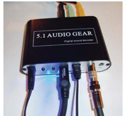
Here, the 5.1 Audio Gear digital sound decoder is on and working. There are three stereo 1/8-inch plug jack cables connected to the jacks on the other end of the decoder that bring the six sound channels out to the amplifiers and speakers. The power-supply cable is the connection on the left; the audio coaxial is the connection on the far right.
