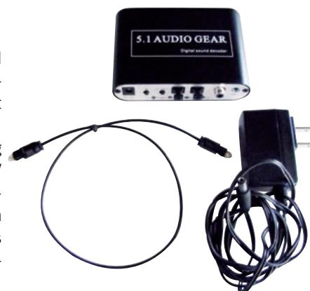
The HD digital 5.1 Audio Gear decoder is small and decodes digital soundtracks out to a set of six speakers.
