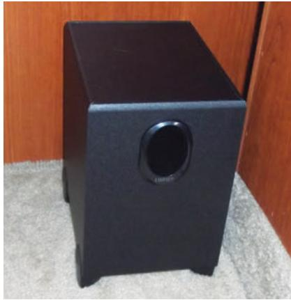
**The LFE speaker can be placed on the floor near the listener and its sound vibrations will be felt as much as heard.**
