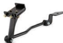
**TIGERTRAK™** Long parabolic springs and extended rear overhang cause gas motorhomes to sway from side-to-side. Placing TIGERTRAK™ between the rear axle and the frame allows unhindered up and down movement of the springs, virtually eliminating tail wag.
