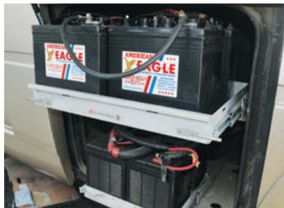
**Building a battery bank that will meet the demands of the individual owner will usually be dictated by the available space to mount the batteries. Here, two slide-out trays can handle four batteries. It's important to have access to the batteries for maintenance and enough clearance to remove caps to replenish flooded-cell batteries.**
