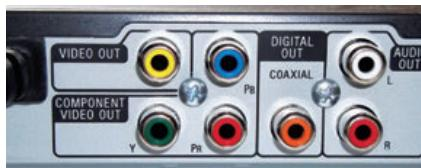
The insulating ring inside of a coaxial RCA output jack is color-coded orange, as shown on the back of this DVD player.
