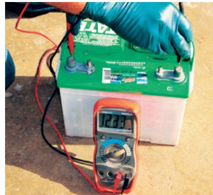
A digital voltmeter, or multimeter, is a great tool. The one shown here is a professional model, but you can find a simple one for around \$20. Touch the probes to the appropriate terminals, and the battery's voltage is displayed on the screen. This one's at 12.33 volts — about 70 percent charged.
